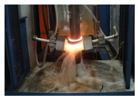
The cooling rate is controlled by adjusting the quench bath temperature or the rate of agitation.
