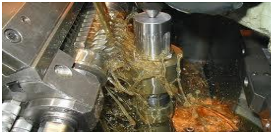
Gear Hobbing operation
